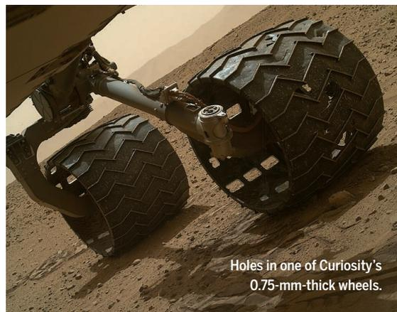
Holes in one of Curiosity's 0.75-mm-thick wheels.
